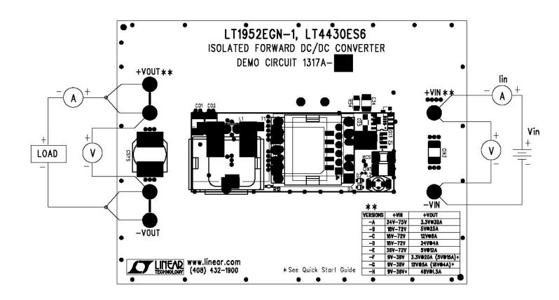
Figure 1. Proper Measurement Equipment Setup
