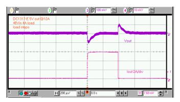
Figure 4. Fast transient response of DC1317A-E is superior to many competing power modules without the additional output capacitors.
