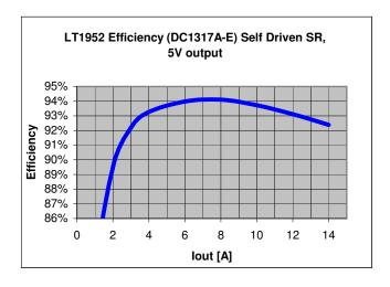
Figure 3. High efficiency of DC1317A-E allows the board to be used in thermally demanding applications
