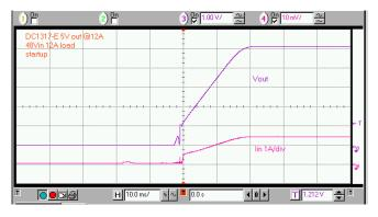
Figure 5. The LT4430 opto coupler driver produces monotonic output voltage rise at startup without output voltage overshoot.
